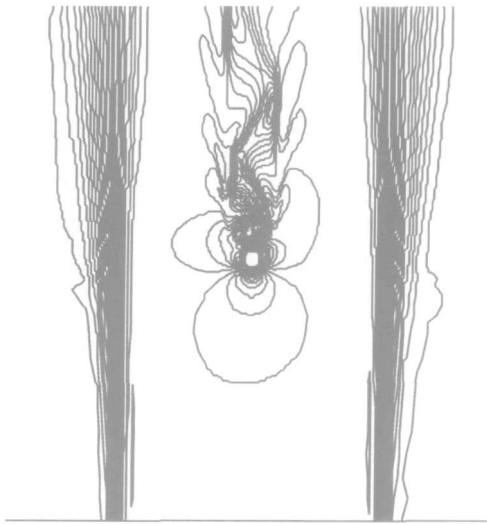
Fig. 11 Mach number distribution for Ma_{in} = 0.4 in free jet flow with B = 0.06
